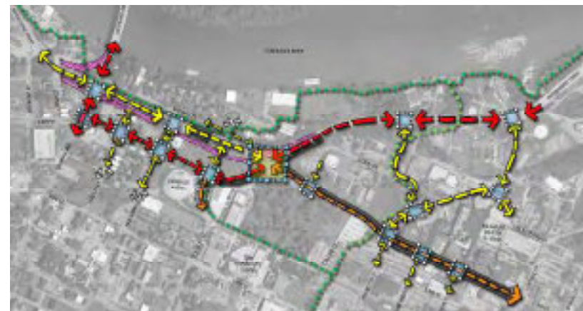
OPTION 2A — MAJOR INTERSECTION This concept provides for a full intersection at Riverfront Parkway and 3rd and 4th Streets. The number of lanes on Riverfront Parkway, 3rd Street and 4th Street vary between two options that are being explored.
