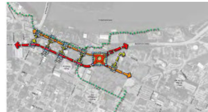
OPTION 3 — ROUNDABOUT The roundabout concept would function similar to the major intersection concept, but would provide continuous flow of traffic between Riverfront Parkway, 3rd Street and 4th Street.
